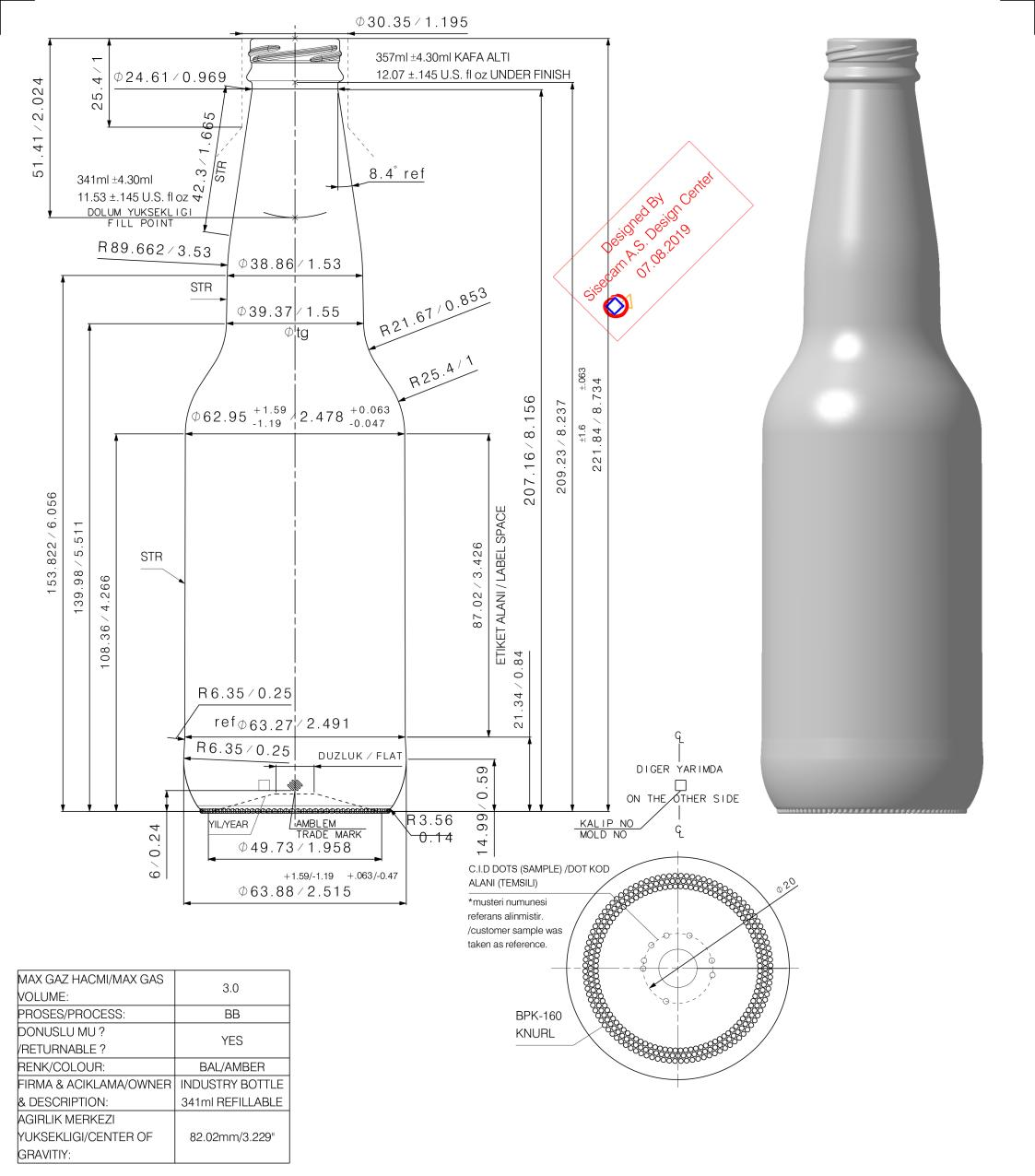
ZORUNLU METIN/MANDATORY TEXT: THIS BOTTLE, AS DESIGNED, DOES NOT PROVIDE STANDARD CROWN REST PLATFORM CLEARANCE. CUSTOMER MUST CONTACT THE EQUIPMENT SUPPLIER TO CONFIRM THAT SUITABLE CLEARANCE IS AVAILABLE.
